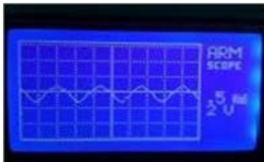
Figure 6.3: 2V and 1KHz Triangular Wave
