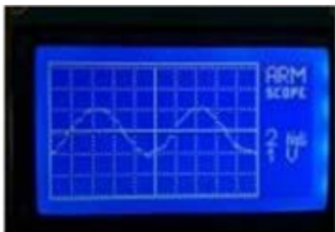
Figure 6.1: 2V and 100Hz Sinosodal Wave
