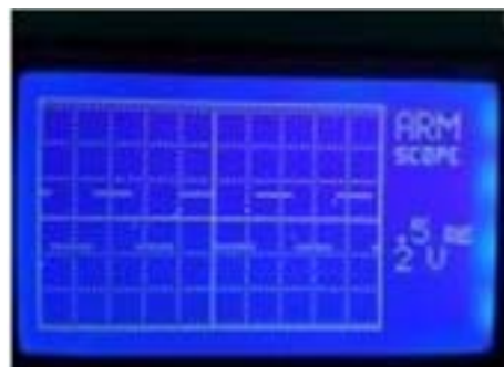
Figure 6.2: 3V and 1KHz Square Wave
