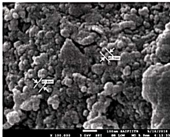
Fig. 3: SEM image of Nanocrystalline \text{CoAl}_2\text{O}_4 thick film.
