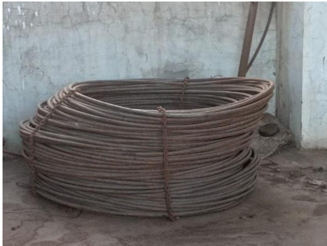
This is round bundle of iron rods 12mm -22mm of pin beeded bundle
