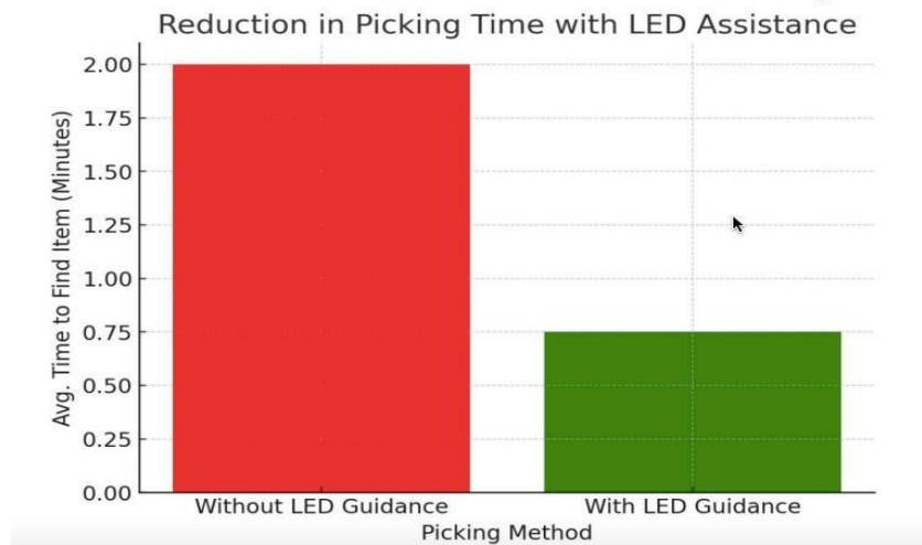
Figure 5.4 Reduction in Picking time with LED Assistance
